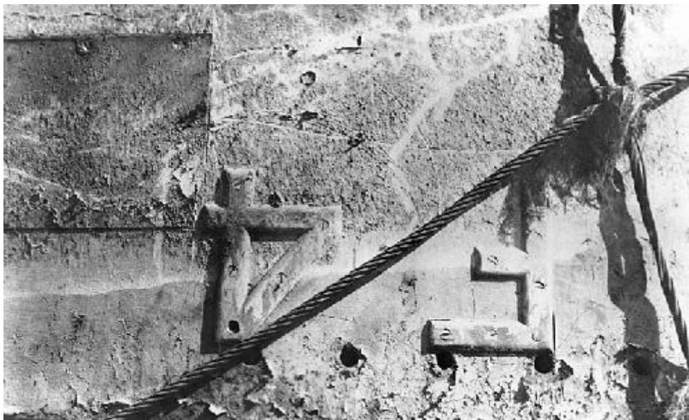
(2) View of F-4's port side name plate, taken in drydock at Honolulu, Hawaii, circa late August or early September 1915, after she had been raised from over 300 feet of water and towed into port. These figures are mounted on the submarine's port bow, and are shown upside down, as she was dry-docked rolled to starboard approximately 120 degrees from the vertical.
